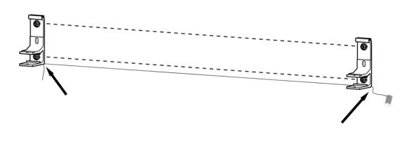
10) Slide the awning (cassette) on wall brackets so that the construction is maximally pressed to the back (Note – before placing the awning verify the alignment of brackets – wall surface should be of the same thickness at installation spots).
