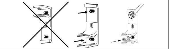
6) Based on the first installed bracket (base) mark installation places for remaining ones – pay paticular attention so that brackets are installed at the same horizontal level and in the same plane.
