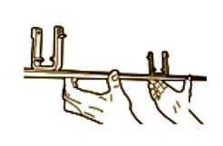
16) Fasten the masking frame profile with brackets to the square bar 40x40 using M8x70 screws.
